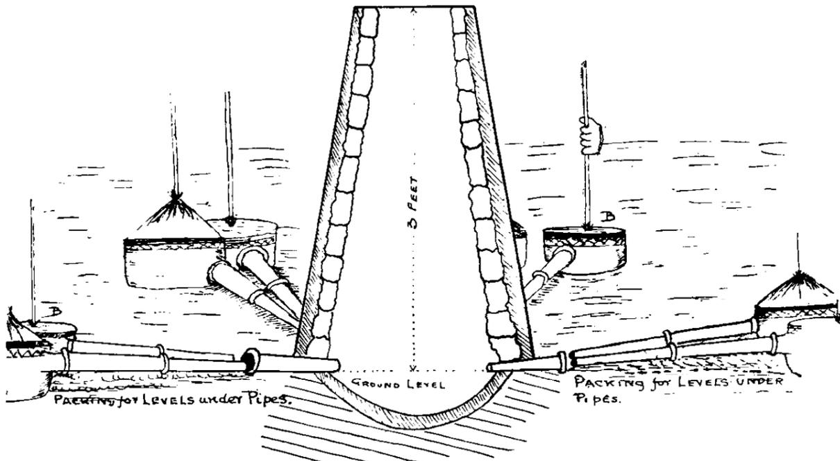
NOTE. As the bellows have no valves the Blast pipe is not connected with the bellows pipes.
