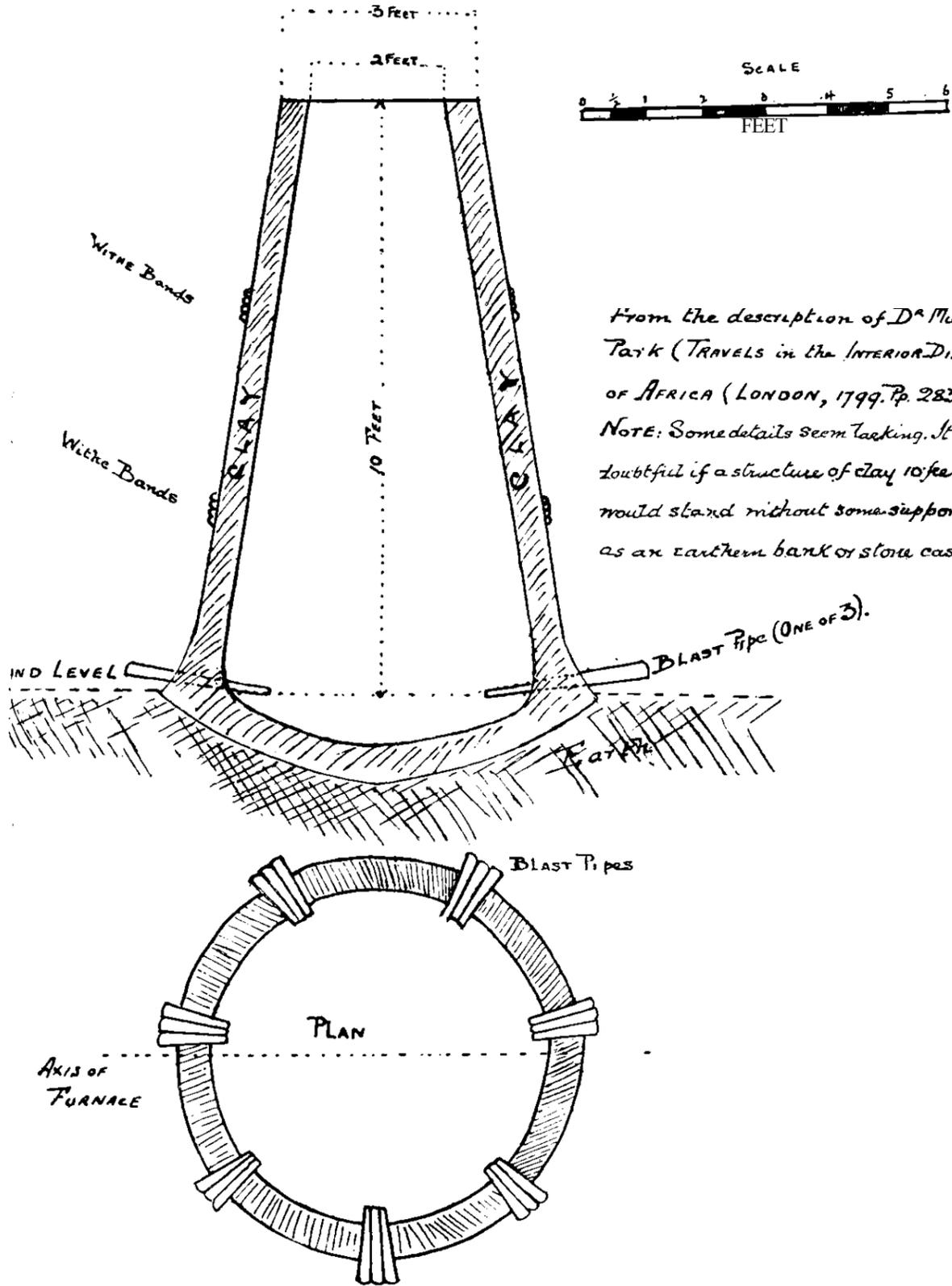
From the description of D<sup>r</sup> Mungo Park (TRAVELS in the INTERIOR-DISTRICTS OF AFRICA (LONDON, 1799. Pp. 283-5. NOTE: Some details seem lacking. It is doubtful if a structure of clay 10 feet high would stand without some support such as an earthen bank or stone casing. A.E.R.
